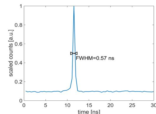
Fig. 6. Instrument response function on a BLUE pixel, 600 nm excitation
