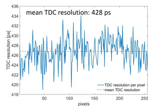
Fig. 3. Time-to-digital converter (TDC) resolution
