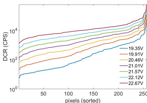
Fig. 2. Dark count rate (DCR) of RED pixels at different bias levels
